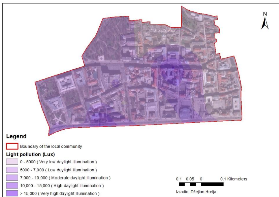
Fig. 3. Map of Illumination in the Morning Hours on a Weekday (Trg Oslobođenja - Centar)
